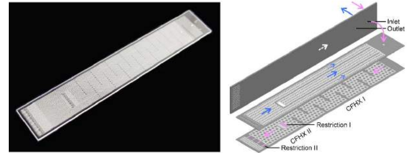
Figure 5 Photograph of the cooler with parallel two-stage expansion (left) and exploded view of the cooler (right). The cooler has a size of 60 x 9.5 x 0.72 mm 3 .
