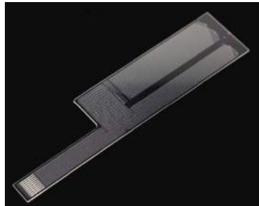
Figure 6 Photograph of the two-stage cooler (left) and exploded view of the cooler (right). The cooler has a size of 90 \times 20.5 \times 0.72 \text{ mm}^3 .
