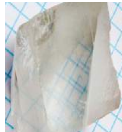
Double refraction in a calcite crystal
